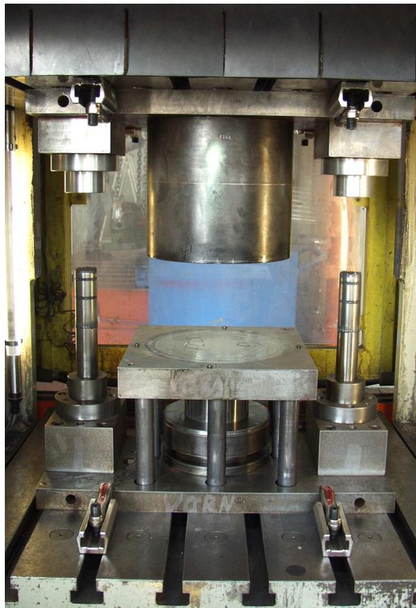
Figure 1: Cup drawing tool setup
