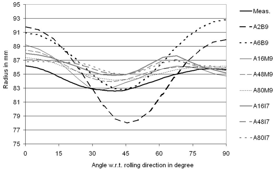
Figure 9: Earing profile for models with ISO12 background and isotropic von Mises component (DX53)
