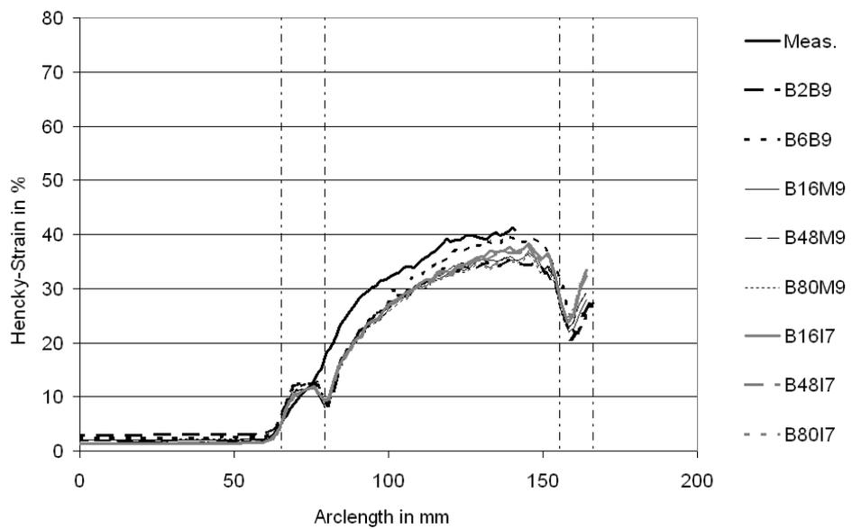
Figure 14: Major strain in rolling direction (ISO12 background, H340)
