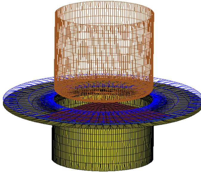
Figure 3: FEM model for the deep drawing simulation
