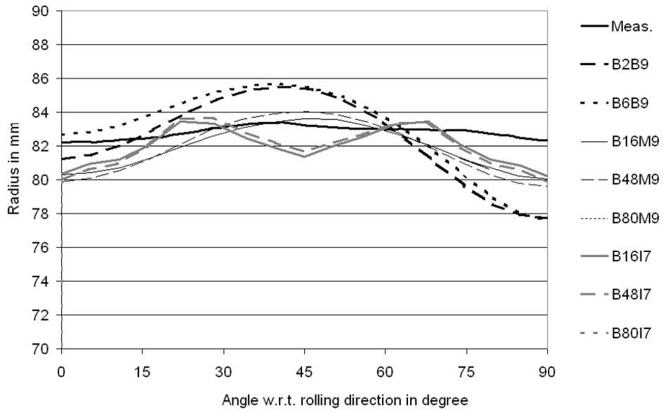
Figure 17: Earing profile for models with ISO12 background and isotropic von Mises component (H340)
