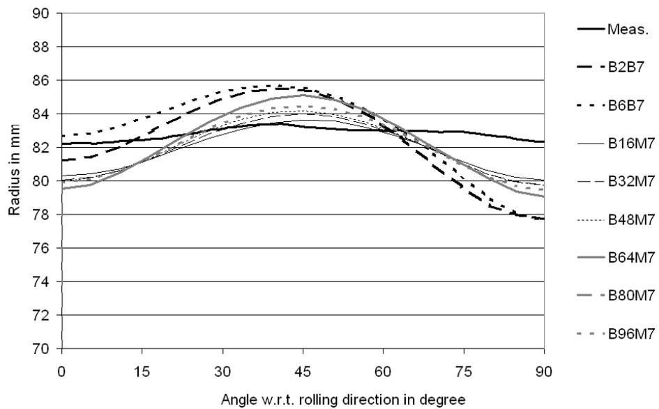
Figure 16: Earing profile for models with isotropic von Mises component (H340)
