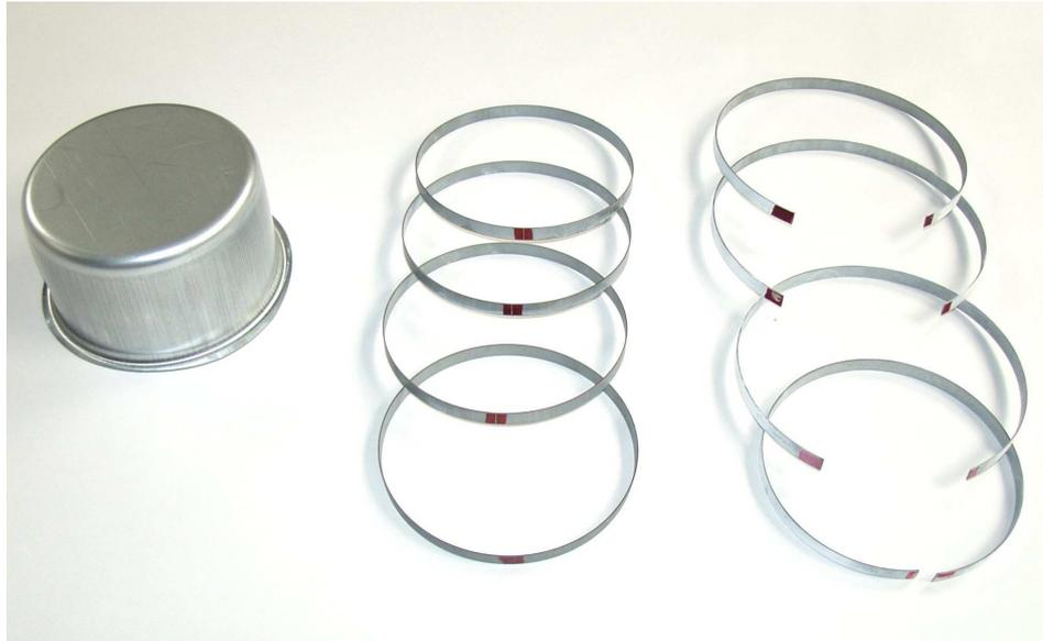
Figure 2: Springback experiment: cup, rings, open rings
