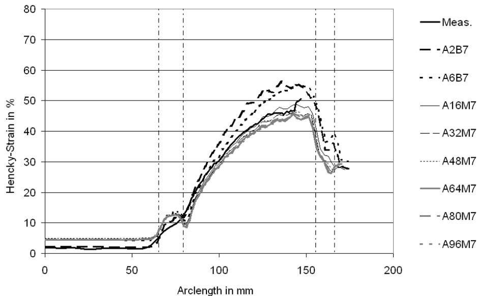
Figure 4: Major strain in rolling direction (isotropic von Mises component, DX53)
