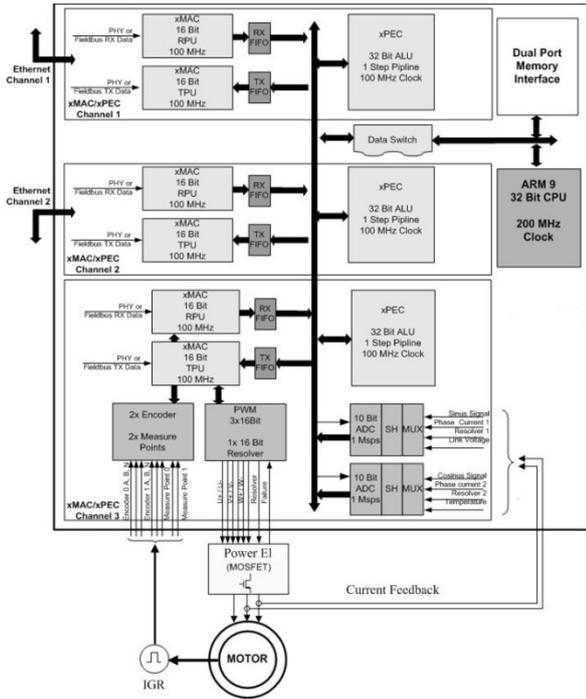
Figure 8. Decentralize Single-Chip controller based on netX processor.
