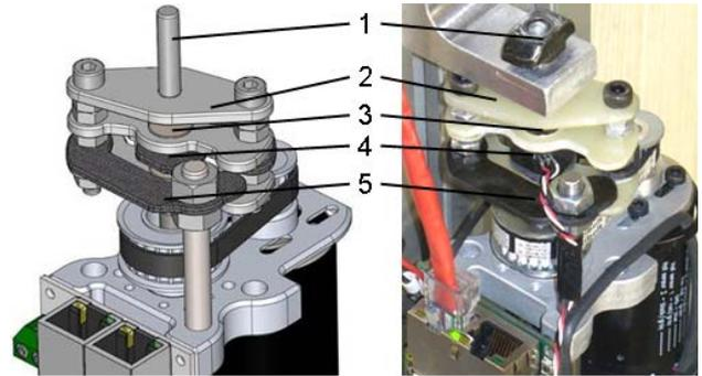
Figure 4. The CAD Model of the elastic actuator (left) and actuator of the robot (right).
