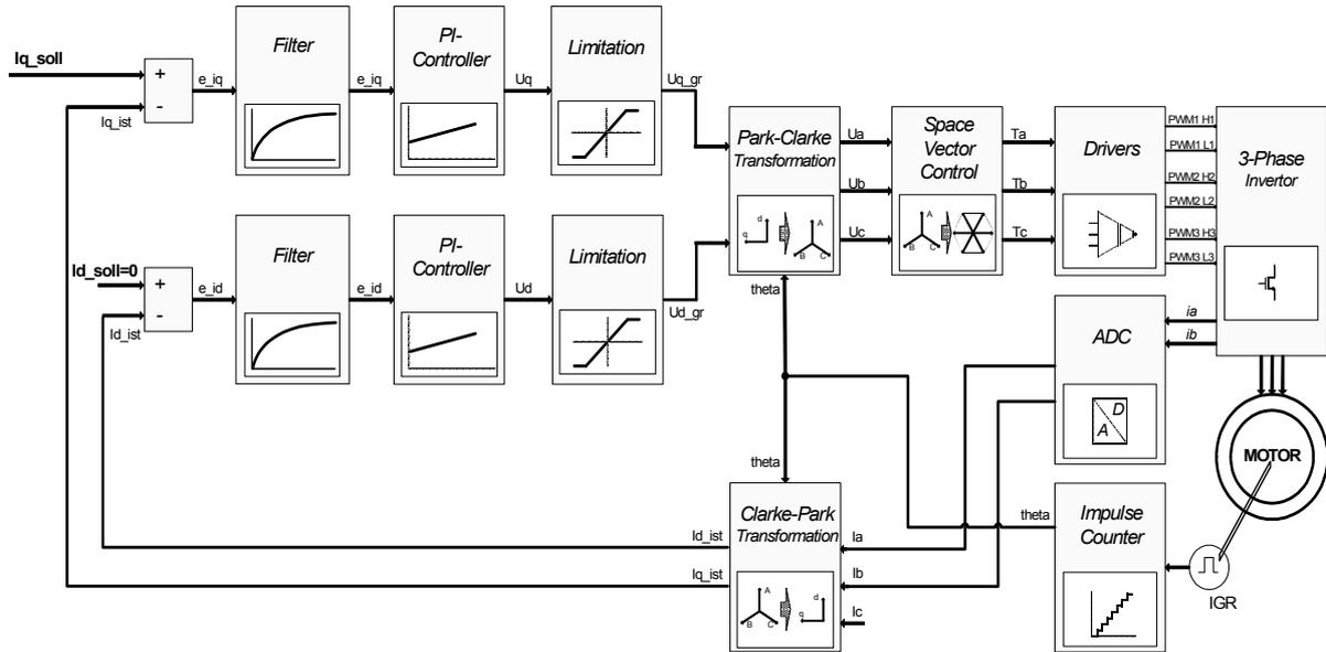
Figure 9. Current control loop in the netX/xPEC.
