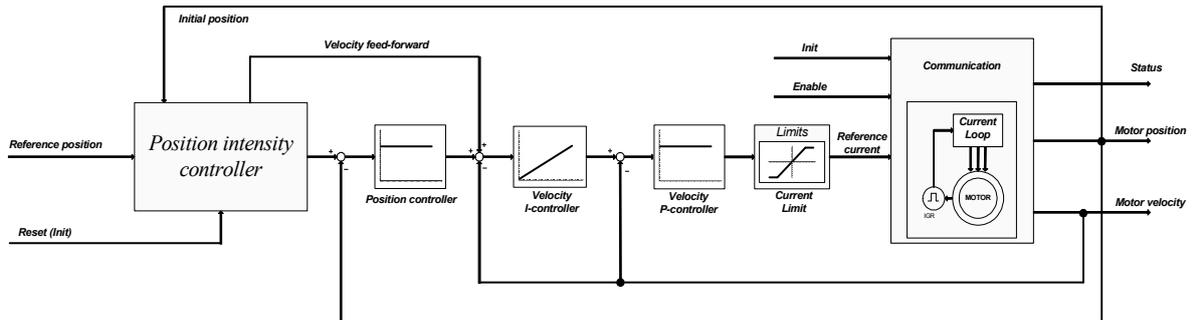
Figure 10. Position/velocity control loops.
