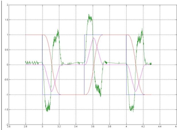
Figure 12. Experimental results: blue – reference position ( $\pm 10$  revolutions); red – actual position ( $\pm 10$  revolutions); magenta – velocity ( $\pm 13000$  rpm); green – current ( $\pm 3.6A$ ).
