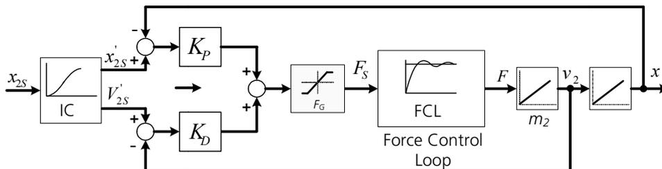
Figure 14. The position control loop.
