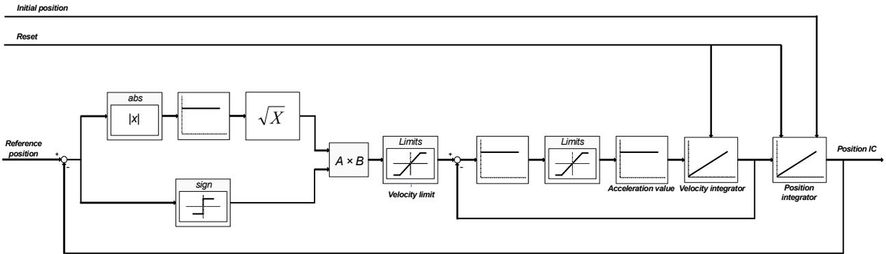
Figure 11. Position intensity controller.
