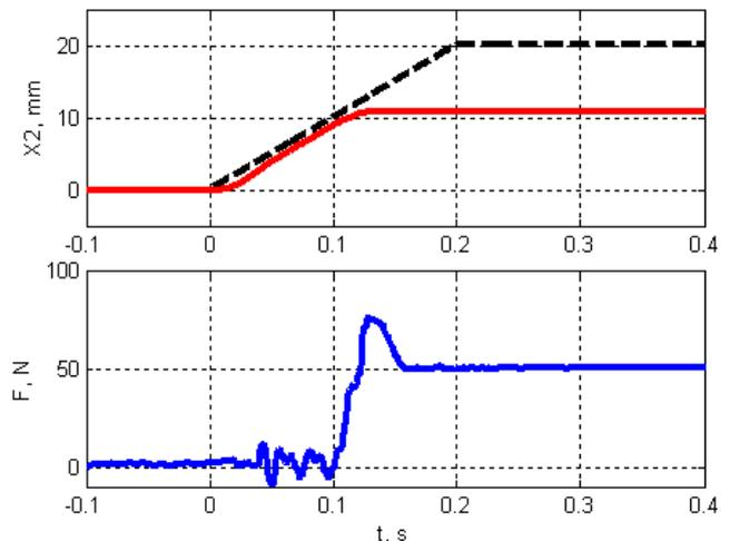
Figure 16. Impact with an obstacle by position control: dotted line – desired position; red line – actual position; blue line – force in the contact.
