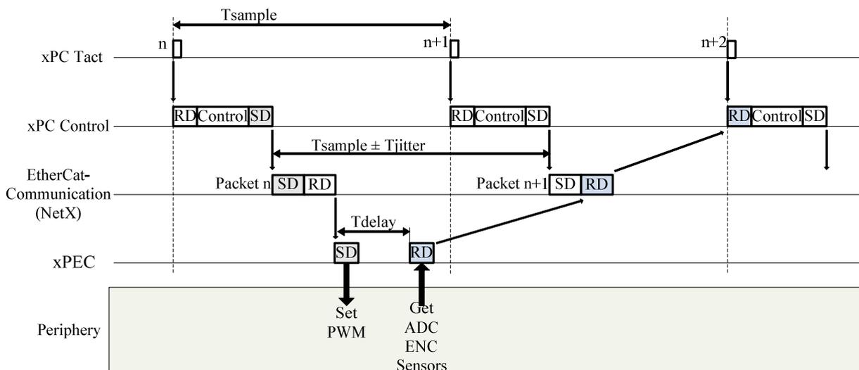
Figure 7. Time diagram of communication process.
