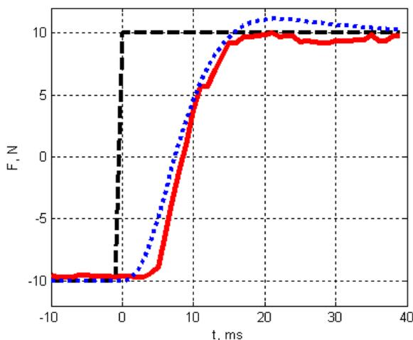
Figure 15. Step response of the force control loop: dotted line – modelling; solid line – experiment.
