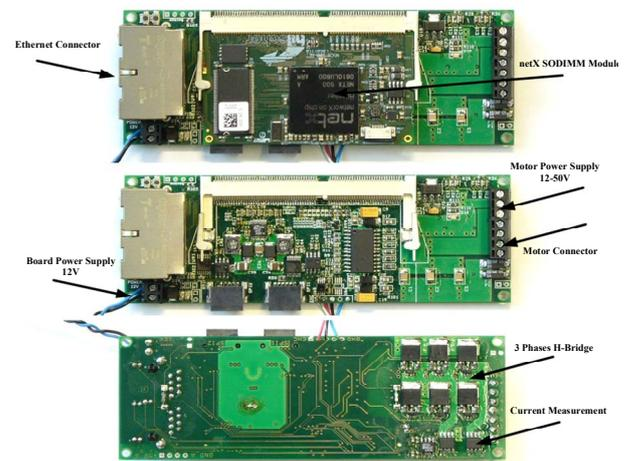
Figure 5. Decentralize control electronics of the biped robot "ROTTA".
