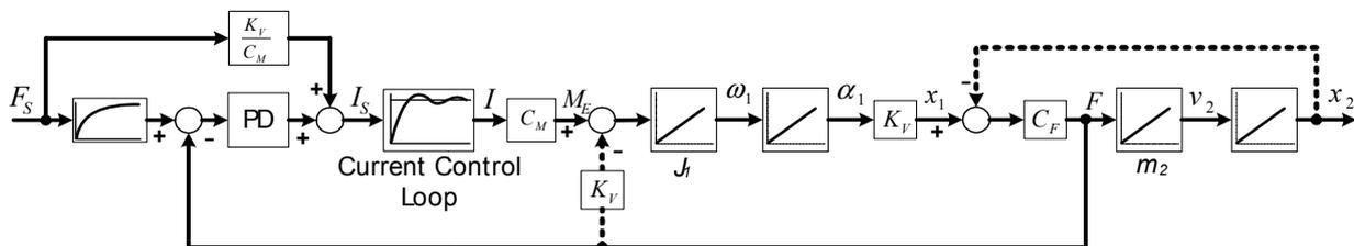
Figure 13. Structural scheme of the force control system, where  $C_F$  – the coefficient of the spring rigidity (spring constant),  $K_V$  – coefficient of the conversion of the rotational motion into the translational motion,  $C_M$  – coefficient of the conversion from current to mechanical torque.
