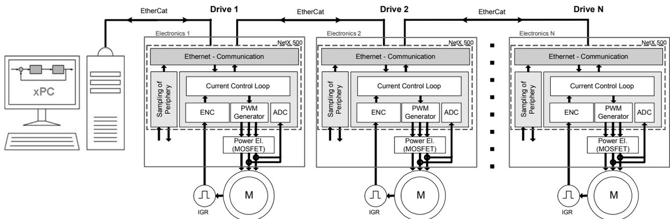
Figure 6. Flexible communication system based on netX processors.
