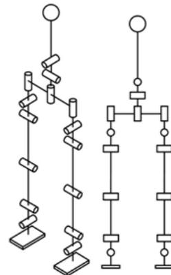
Figure 1. Kinematic structure of biped robot "ROTTA".
