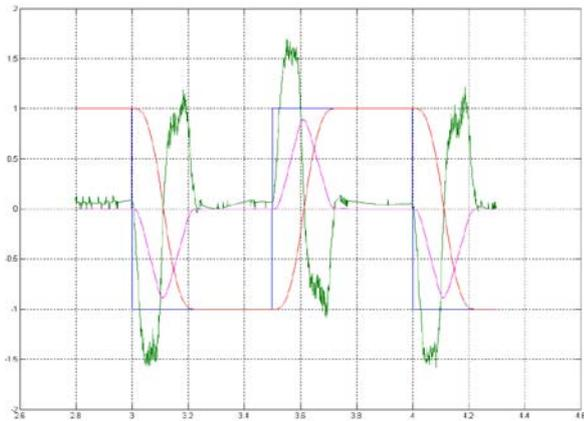
**Figure 10** Experimental results: blue – reference position ( $\pm 10$  revolutions); red – actual position ( $\pm 10$  revolutions); magenta – velocity ( $\pm 13000$  rpm); green – current ( $\pm 3,6A$ )
