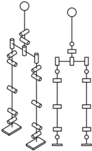
**Figure 1** Kinematic structure of biped robot “ROTTA”
