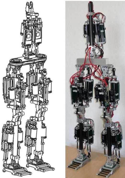
**Figure 2** CAD construction (left); real biped robot “ROTTA” (right)
