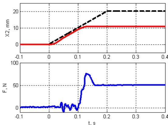
**Figure 14** Impact with an obstacle by position control: dotted line – desired position; red line – actual position; blue line – force in the contact
