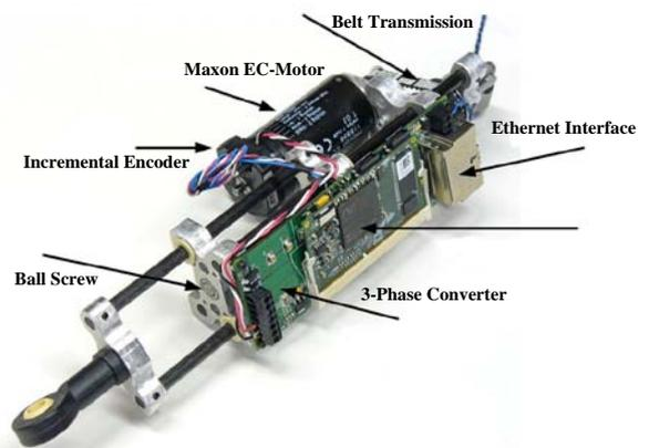
**Figure 3** Linear actuator of biped robot “ROTTA”
