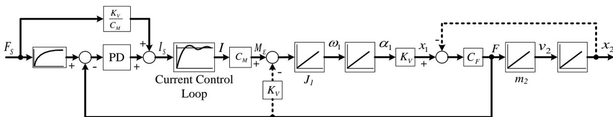
**Figure 11** Structural scheme of the force control system, where  $C_F$  – the coefficient of the spring rigidity (spring constant),  $K_V$  – coefficient of the conversion of the rotational motion into the translational motion,  $C_M$  – coefficient of the conversion from current to mechanical torque
