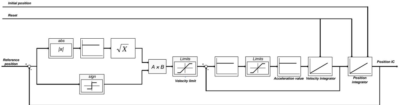
**Figure 9** Position intensity controller
