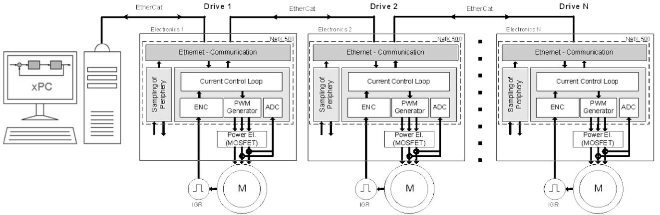
**Figure 5** Flexible communication system based on netX processors
