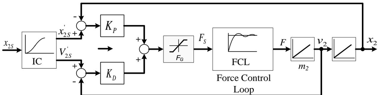
**Figure 13** The position control loop
