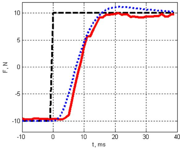
**Figure 12** Step response of the force control loop: dotted line – modelling; solid line – experiment
