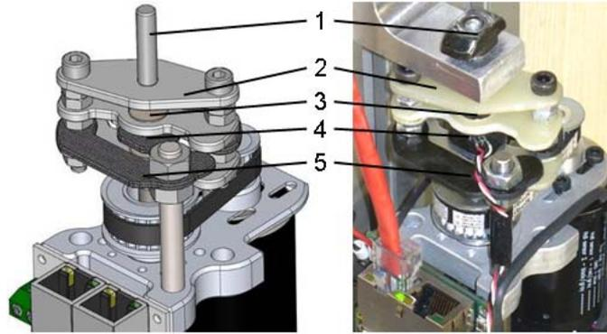
Figure 1. The CAD Model of the elastic actuator (left) and actuator of the robot (right).
