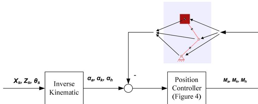
Figure 9. Position control system of robot's leg.
