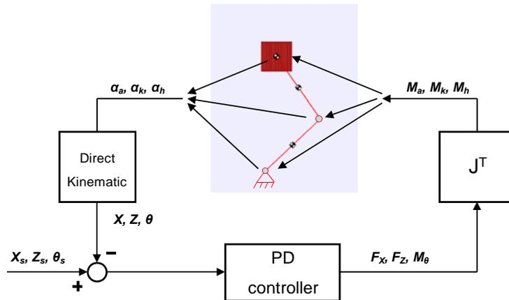
Figure 8. Position control system of robot's leg based on approach of "Virtual Force Control".
