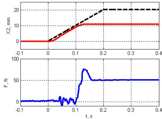
Figure 5. Impact with an obstacle by position control: dotted line – desired position; red line – actual position; blue line – force in the contact.
