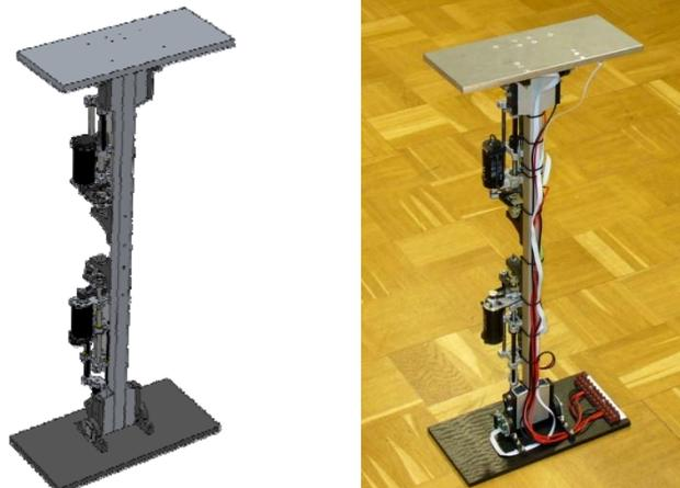
Figure 5. 2D 2-DOF robot's leg.
