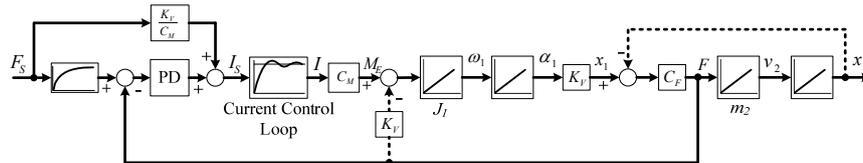
Figure 2. Structural scheme of the force control system, where  $C_F$  – the coefficient of the spring rigidity (spring constant),  $K_V$  – coefficient of the conversion of the rotational motion into the translational motion,  $C_M$  – coefficient of the conversion from current to mechanical torque.
