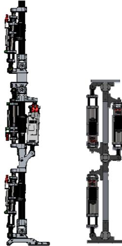
Figure 6. Real two legged robot "ROTT0" (left) and simple 2D robot's leg (right).
