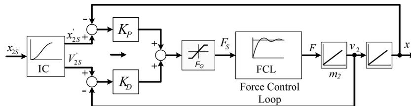
Figure 4. The position control loop.
