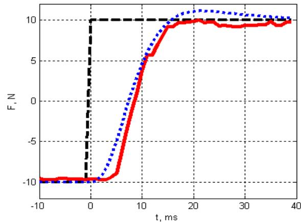
Figure 3. Step response of the force control loop: dotted line – modelling; solid line – experiment.
