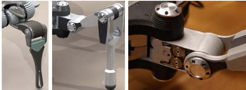
Figure 2. Constructions of legs and the shoulder’s differential joints (SLAIR2, ANTON, real differential joint on robot “ANTON”).
