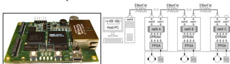
Figure 2. Flexible communication system based on netX processors.
